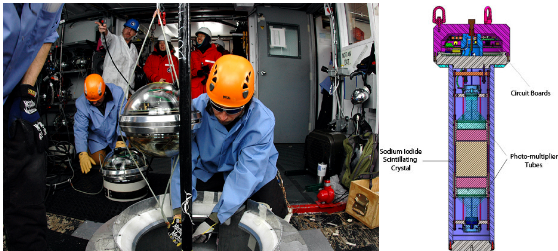
Figure 2. Two pressure-hardened physics experiments deployed in hot-water-drilled holes in the South Pole ice cap in 2010. Left: IceCube experimenters deploying a string of photomultiplier tube modules (DOMs). Photo credit Peter Rejcek. Right: Schematic of DM-ICE prototype dark matter detector. Drawing courtesy Physical Sciences Laboratory, Wisconsin
